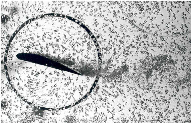
Figure 1: Bubbly flow around a NACA 4412 hydrofoil (10cm chord) at an angle of attack; flow is from left to right. From the work of Ohashi *et al.*, reproduced with the author's permission.
