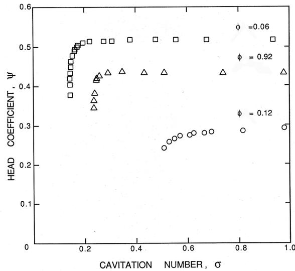
Figure 4: Cavitation performance for a typical centrifugal pump (Franz *et al.* 1990) for three different flow coefficients,  $\phi$
