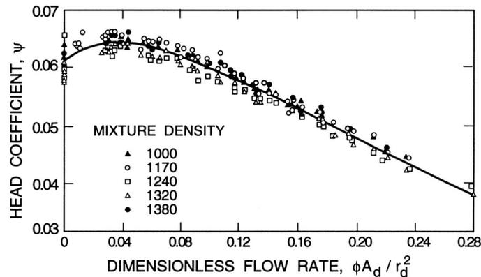
Figure 1: The head coefficient,  $\psi$ , for a centrifugal dredge pump ingesting silt/clay/water mixtures plotted against a non-dimensional flow rate,  $\phi A_d / r_d^2$ , for various mixture densities (in  $\text{kg/m}^3$ ). Adapted from Herbich (1975).
