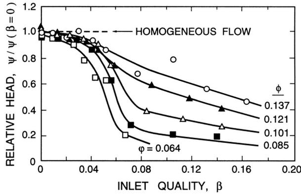
Figure 3: The ratio of the pump head with air/water mixtures to the head with water alone,  $\psi / \psi(\beta = 0)$ , as a function of the inlet volumetric quality,  $\beta$ , for various flow coefficients,  $\phi$ . Data from Patel and Runstadler (1978) for a centrifugal pump.
