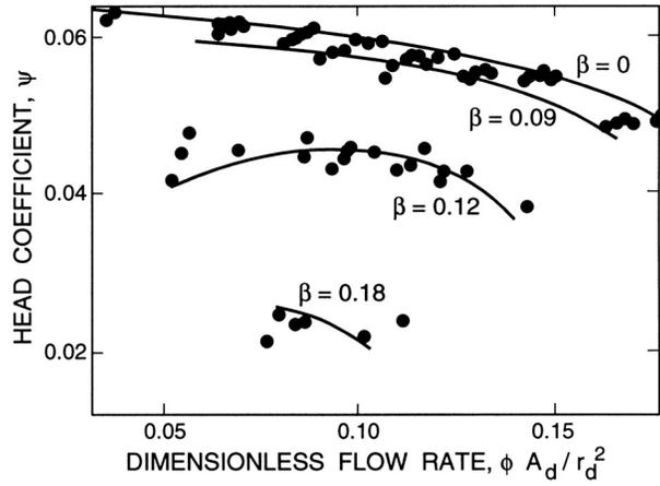
Figure 2: The head coefficient,  $\psi$ , for a centrifugal dredge pump ingesting air/water mixtures plotted against a non-dimensional flow rate,  $\phi A_d / r_d^2$ , for various volumetric qualities,  $\beta$ . Adapted from Herbich (1975).
