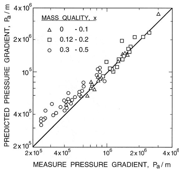
Figure 2: Comparison of the measured friction coefficient with that using the homogeneous prediction for steam/water flows of various mass qualities in a 0.3cm diameter tube. From Owens (1961).
