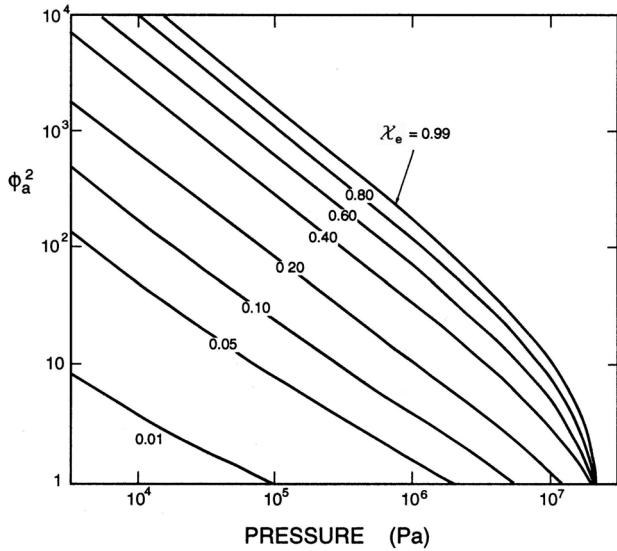
Figure 3: The Martinelli-Nelson acceleration pressure drop function,  $\phi_a^2$ , for water as a function of the prevailing pressure level and the exit mass quality,  $\chi_e$ . Case shown is for  $\kappa_L = \kappa_G = 1.0$  and  $m_L = m_G = 0.25$ .
