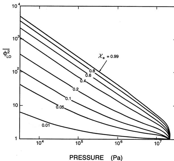
Figure 1: The Martinelli-Nelson frictional pressure drop function,  $\overline{\phi_{L0}^2}$ , for water as a function of the prevailing pressure level and the exit mass quality,  $\mathcal{X}_e$ . Case shown is for  $\kappa_L = \kappa_G = 1.0$  and  $m_L = m_G = 0.25$ .
