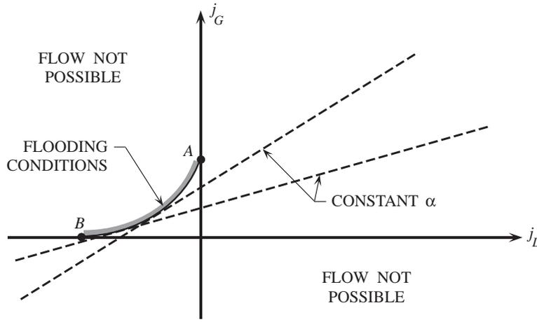
Figure 2: Flooding envelope in a flow pattern diagram.
