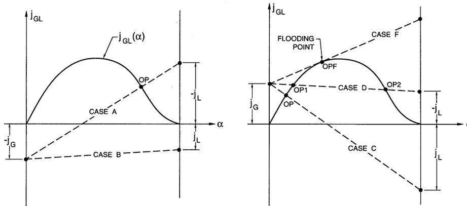
Figure 1: Drift flux charts for the vertical flows of gas-liquid mixtures. Left: for downward gas flux. Right: for upward gas flux.
