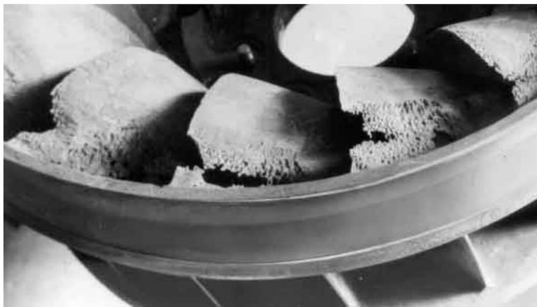
Figure 1: Major cavitation damage to the blades at the discharge from a Francis turbine.
