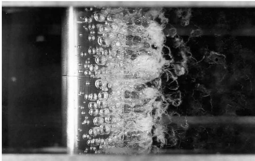
Figure 1: Dense traveling bubble cavitation on the surface of a NACA 4412 hydrofoil at zero incidence angle, a speed of  $13.7\text{ m/s}$  and a cavitation number of 0.3. The flow is from left to right and the leading edge of the foil is just to the left of the white glare patch on the surface (Kermeen 1956).
