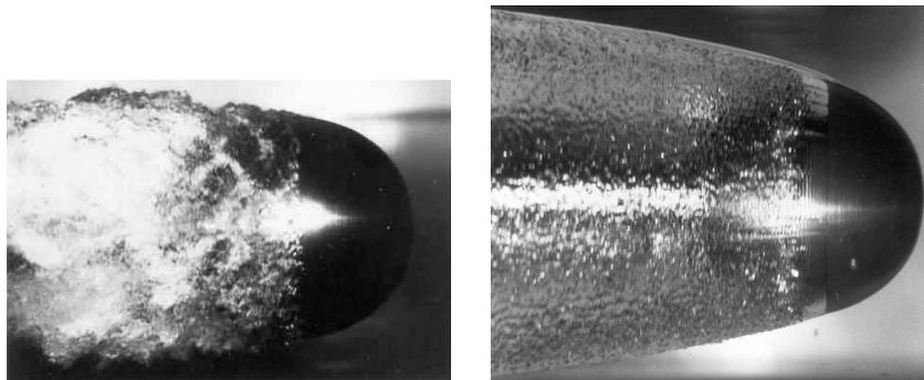
Figure 2: Two photographs of a cavitating,  $7.62\text{ cm}$  diameter sphere. The left photograph shows bubble cavitation and bubbly wake prior to the transition to the fully developed cavity shown on the right (Brennen 1970). The flow is from right to left, the velocities being  $5.6\text{ m/s}$  and  $10.7\text{ m/s}$ , respectively.
