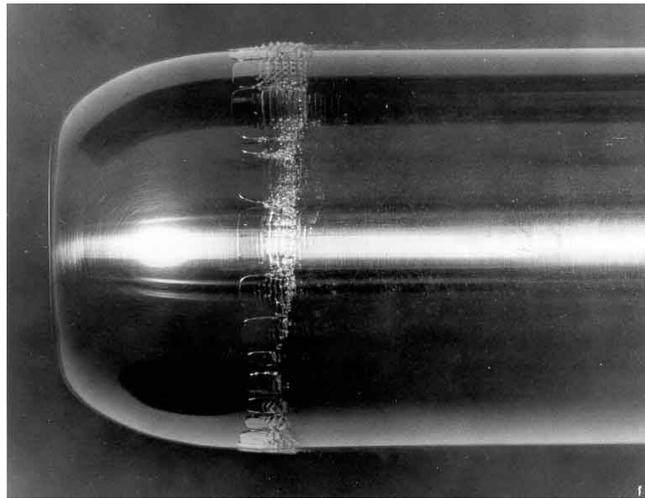
Figure 4: Sheet cavitation on the ITTC headform. The flow is from left to right with a speed of 12.2 *m/s* and a cavitation number of 0.424. Reproduced with the permission of A.J. Acosta.
