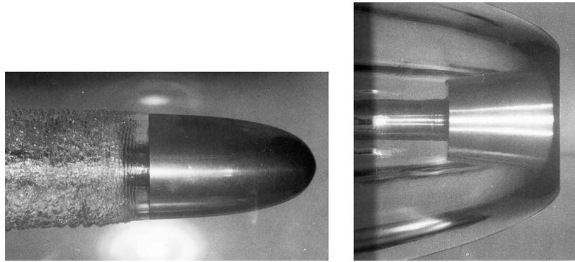
Figure 3: Two fully developed cavities on a 5.95 *cm* diameter ogive (left) and a 7.62 *cm* diameter disc (right) set normal to the oncoming stream (Brennen 1970). The flow is from right to left and the velocities are 7.62 *m/s* and 10.7 *m/s*, respectively.
