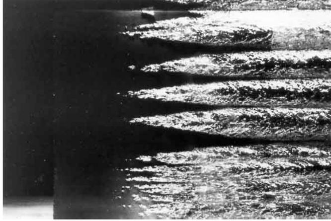
Figure 5: Streak cavitation on a biconvex hydrofoil at a speed of  $15.5 \text{ m/s}$  and a cavitation number of  $0.11$  (Arakeri 1975). The flow is from left to right and the leading edge of the foil is about  $1 \text{ cm}$  from the left-hand edge. Reproduced with the permission of V.H. Arakeri.
