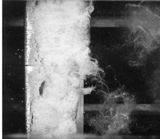
Figure 1: Sheet cavitation on the suction surface of a NACA 4412 hydrofoil at an angle of attack of  $12^\circ$ , a speed of  $10.7\text{ m/s}$  and a cavitation number of 1.05 (Kermeen 1956). The flow is from left to right.
