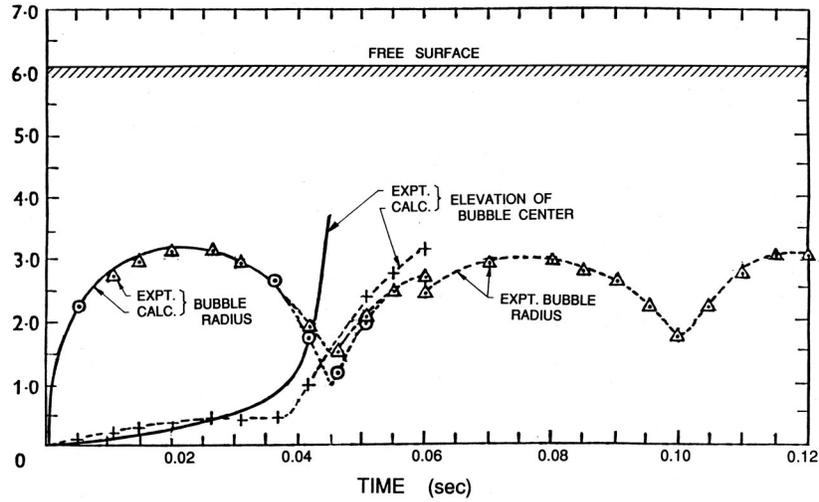
Figure 2: Data from Davies and Taylor (1943) on the mean radius and central elevation of a bubble in oil generated by a spark-initiated explosion of  $1.32 \times 10^6$  ergs situated 6.05 cm below the free surface. The two measures of the bubble radius are one half of the horizontal span ( $\Delta$ ) and one quarter of the sum of the horizontal and vertical spans ( $\odot$ ). Theoretical calculations using equation (Nff3) are indicated by the solid lines.
