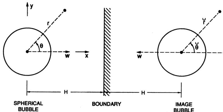
Figure 1: Schematic of a bubble undergoing growth or collapse close to a plane boundary. The associated translational velocity is denoted by  $W$ .
