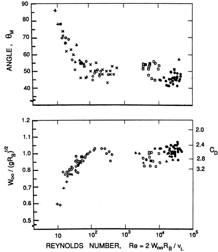
Figure 2: Data on the terminal velocity,  $W_\infty/(gR_B)^{1/2}$ , and the conical angle,  $\theta_M$ , for spherical-cap bubbles studied by a number of different investigators (adapted from Wegener and Parlange 1973).
