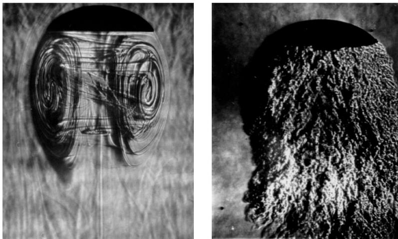
Figure 3: Flow visualizations of spherical-cap bubbles. On the left is a bubble with a laminar wake at  $Re \approx 180$  (from Wegener and Parlange 1973) and, on the right, a bubble with a turbulent wake at  $Re \approx 17,000$  (from Wegener, Sundell and Parlange 1971, reproduced with permission of the authors).
