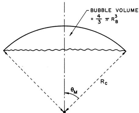
Figure 1: Photograph of a spherical cap bubble rising in water (from Davenport, Bradshaw, and Richardson 1967) with the notation used to describe the geometry of spherical cap bubbles.
