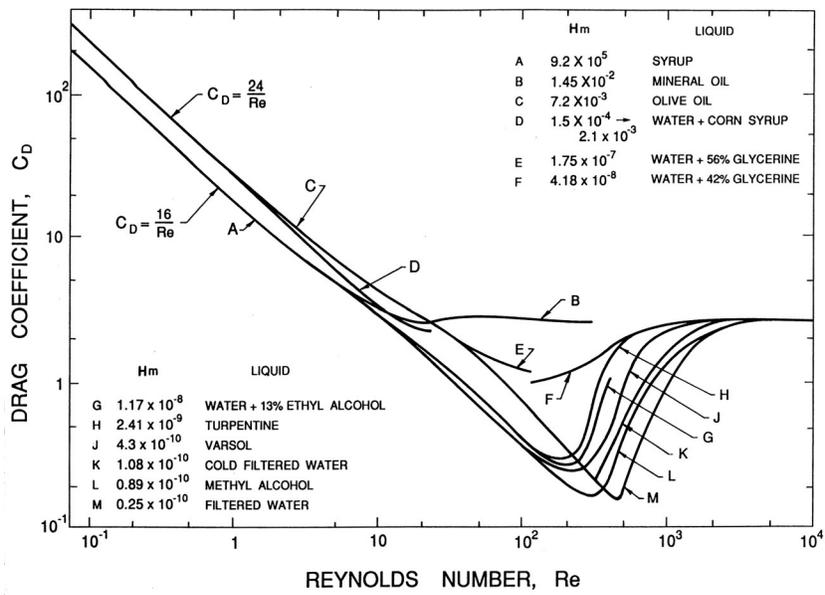
Figure 4: Drag coefficients,  $C_D$ , for bubbles as a function of the Reynolds number,  $Re$ , for a range of Haberman-Morton numbers,  $Hm$ , as shown. Data from Haberman and Morton (1953).
