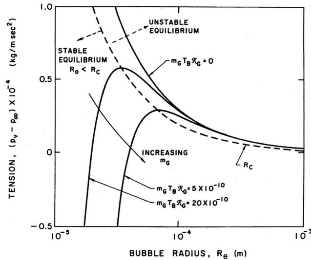
Figure 1: Stable and unstable bubble equilibrium radii as a function of the tension for various masses of gas in the bubble. Stable and unstable conditions are separated by the dotted line. Adapted from Daily and Johnson (1956).
