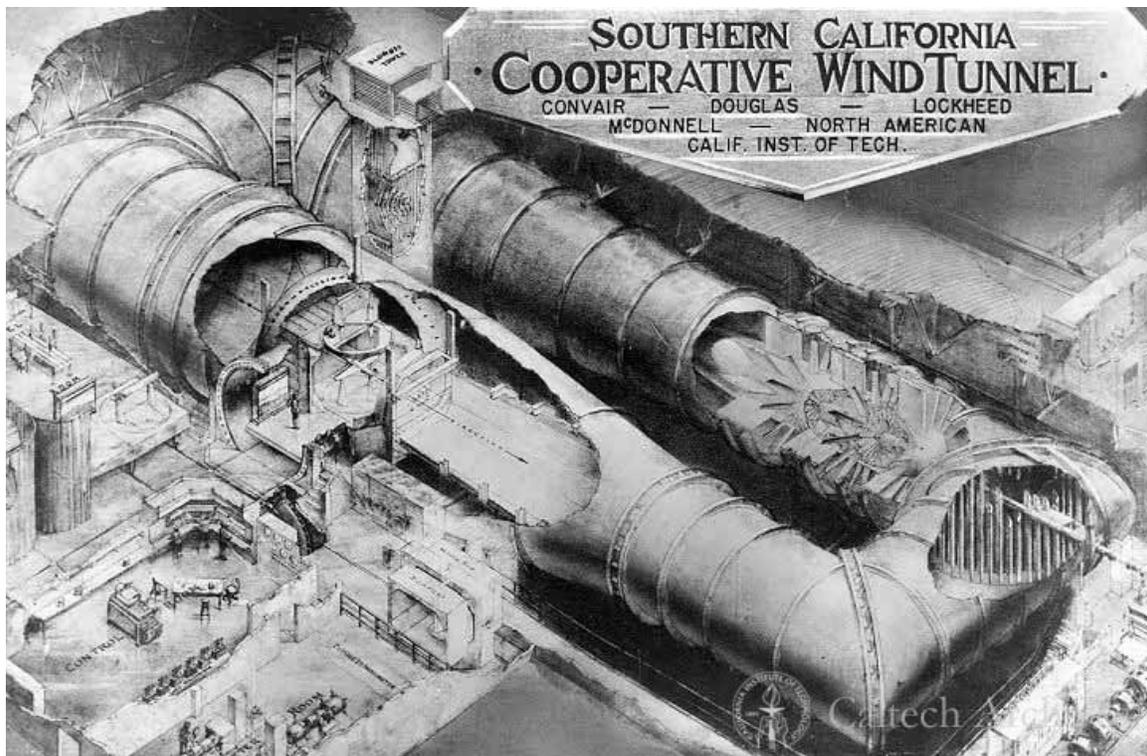
Figure 1: Russell W. Porter schematic of the Southern California Cooperative Wind Tunnel.
