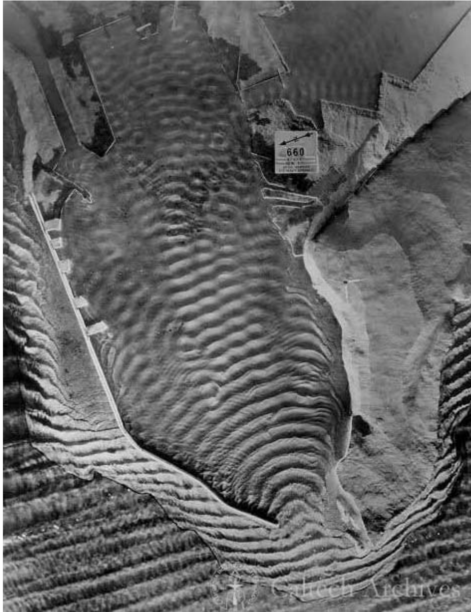
Figure 1: Model basin with a harbor model installed in a study of the harbor wave dynamics.
