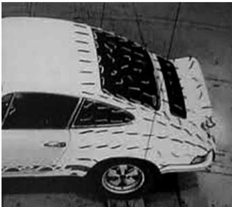
Figure 5: Flow visualization with tufts on an automobile.
