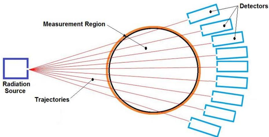
Figure 2: Schematic of a single source, tomographic arrangement deployed around a tube containing a flow.
