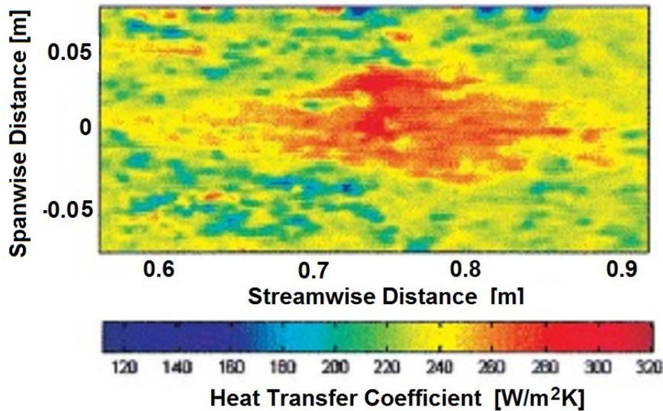
Figure 1: Liquid crystal visualization of the heat transfer and therefore the shear stress under a turbulent spot. Photograph by Guo *et al.* (2000).
