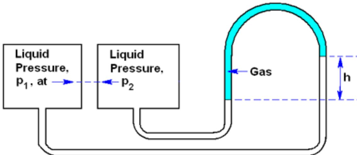
Figure 3: An inverted gas/liquid manometer.
