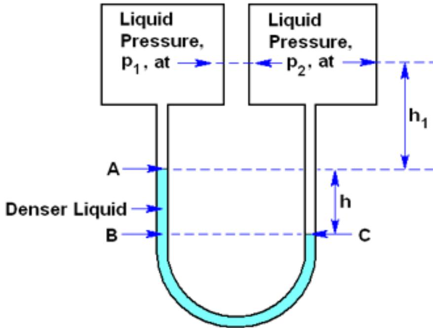
Figure 2: Basic liquid manometer for measuring liquid pressure differences.
