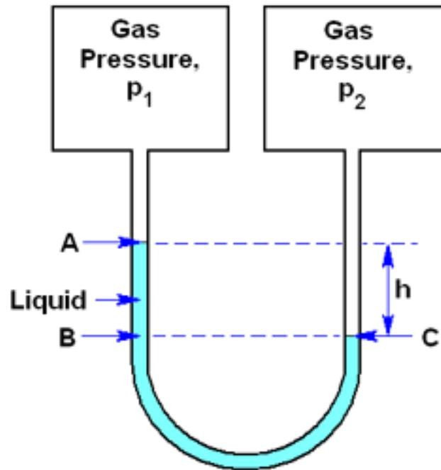
Figure 1: Basic liquid manometer for measuring a gas pressure difference.
