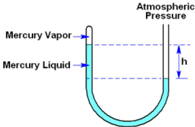
Figure 3: A mercury barometer.
