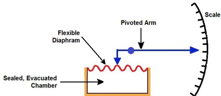
Figure 1: A simple barometer.
