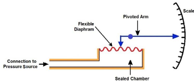
Figure 2: A simple pressure gauge.
