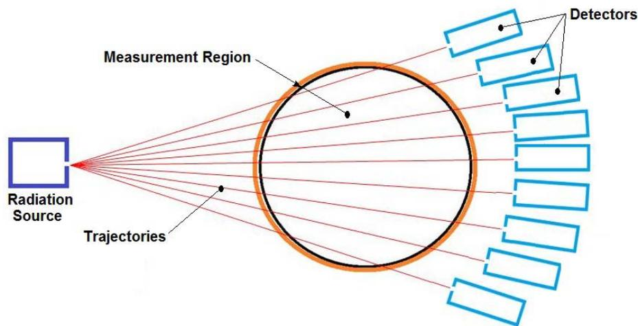
Figure 1: Schematic of a single source, tomographic arrangement deployed around a tube containing a flow.
