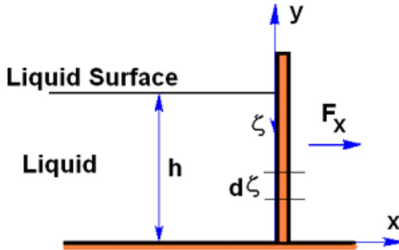
Figure 1: Sketch of a two-dimensional dam and reservoir, depth  $h$ .
