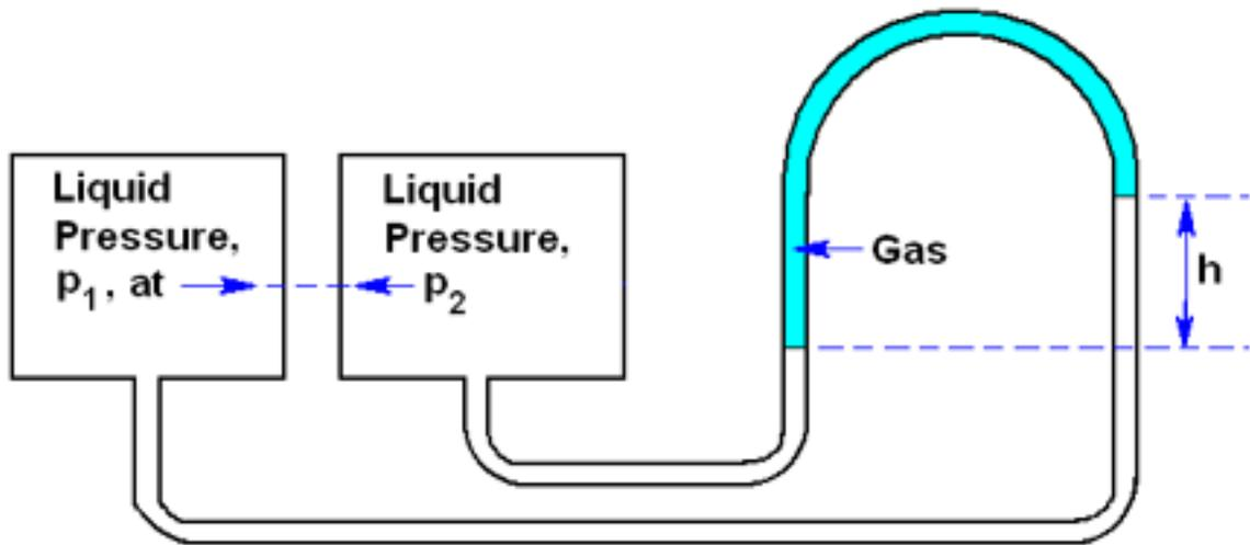
Figure 3: An inverted gas/liquid manometer.
