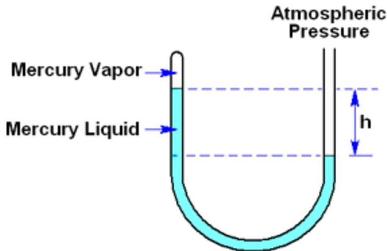
Figure 4: A mercury barometer.
