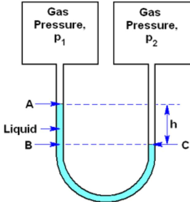
Figure 1: Basic liquid manometer for measuring gas pressure differences.
