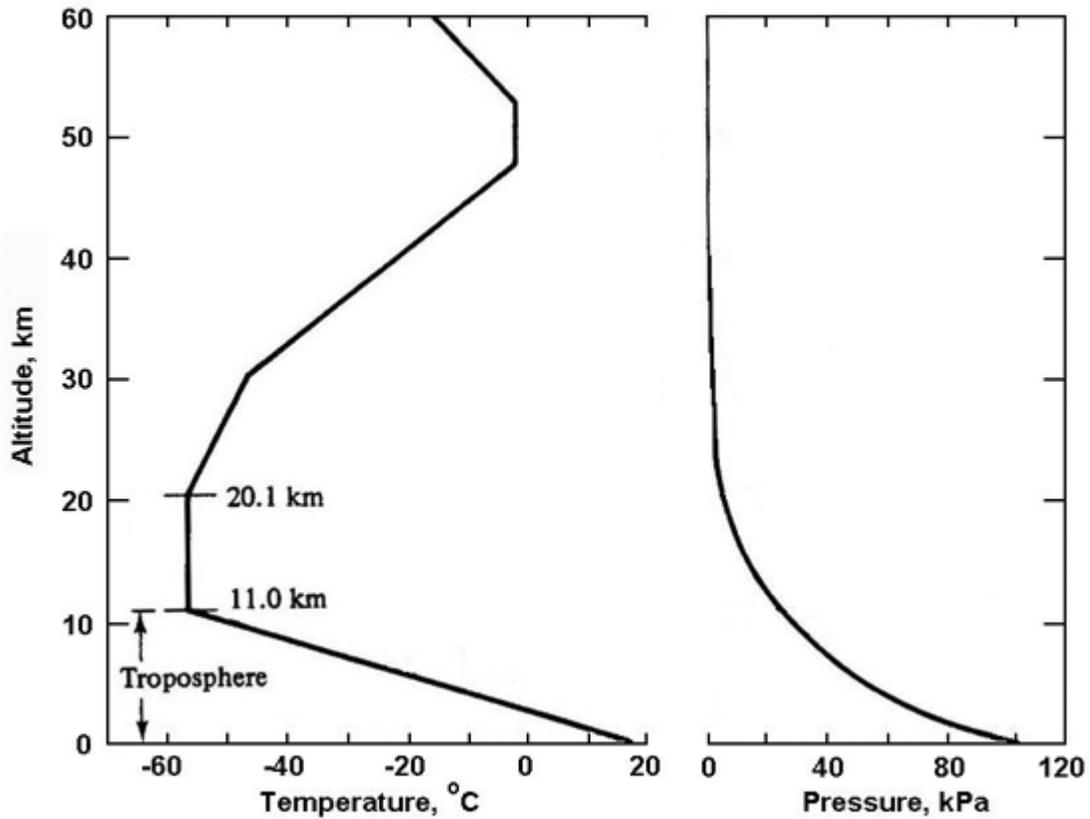
Figure 1: The U.S. standard atmosphere showing the variations in temperature and pressure with altitude.
