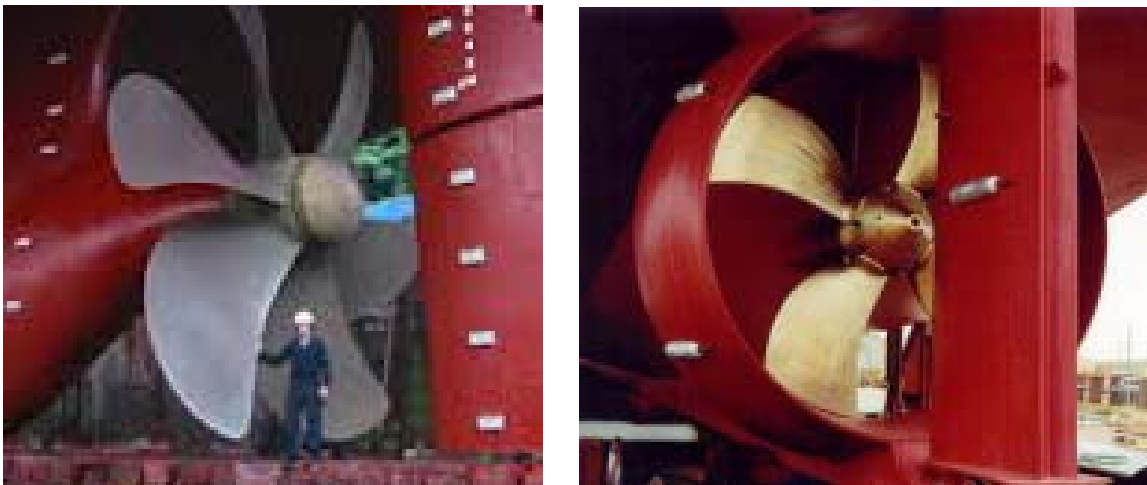
Figure 2: Left: Typical ship propeller. Right: Ducted marine propeller.
