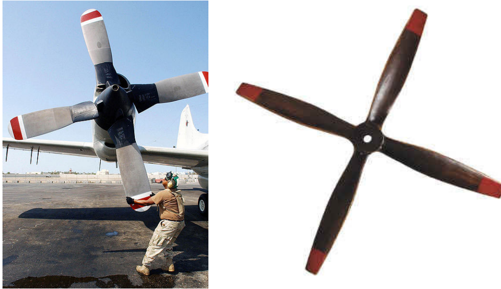
Figure 1: Left: Hamilton Standard 54H60 propeller on US Navy plane. Right: A typical high aspect ratio propeller, AP156-hi.
