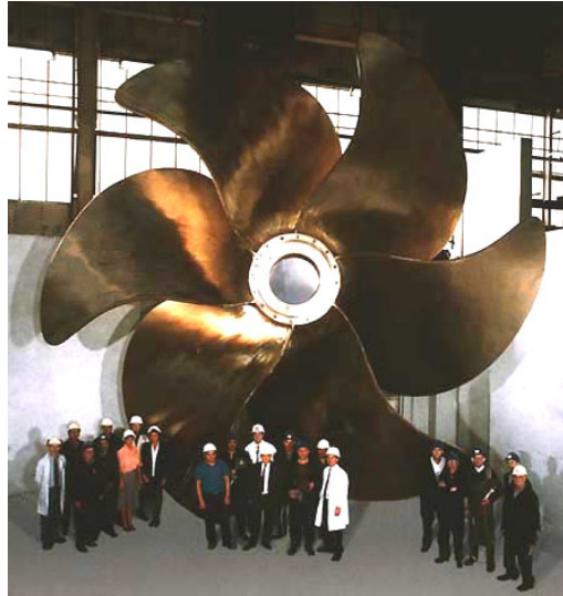
Figure 2: Left: Five different marine propeller designs. Right: 85 ton, bronze marine propeller.
