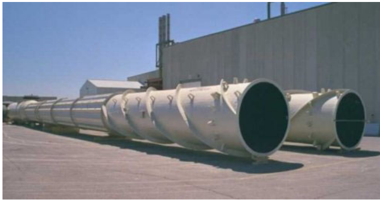
Figure 6: Fins on large industrial chimney.
