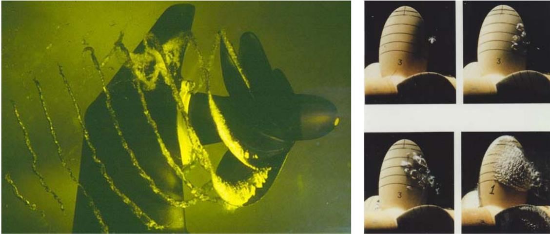
Figure 2: Examples of cavitation on marine propellers.
