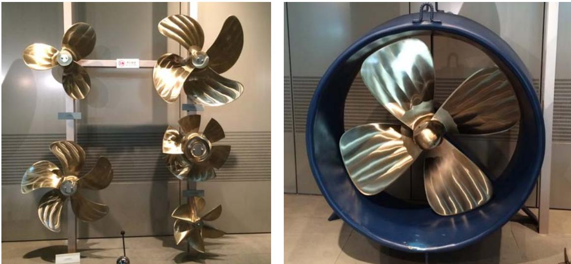
Figure 3: Left: Five different marine propeller designs. Right: Ducted marine propeller.
