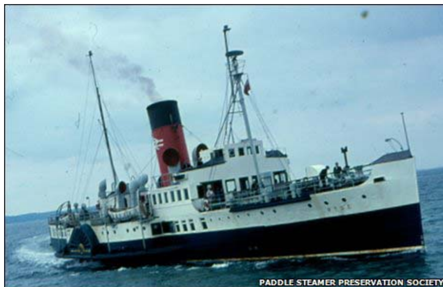
Figure 2: Paddle steamer "Ryde", a typical sidewheeler, built on the River Clyde by William Denny and Brothers and launched in April 1937. She saw service as a ferry for over 30 years.
