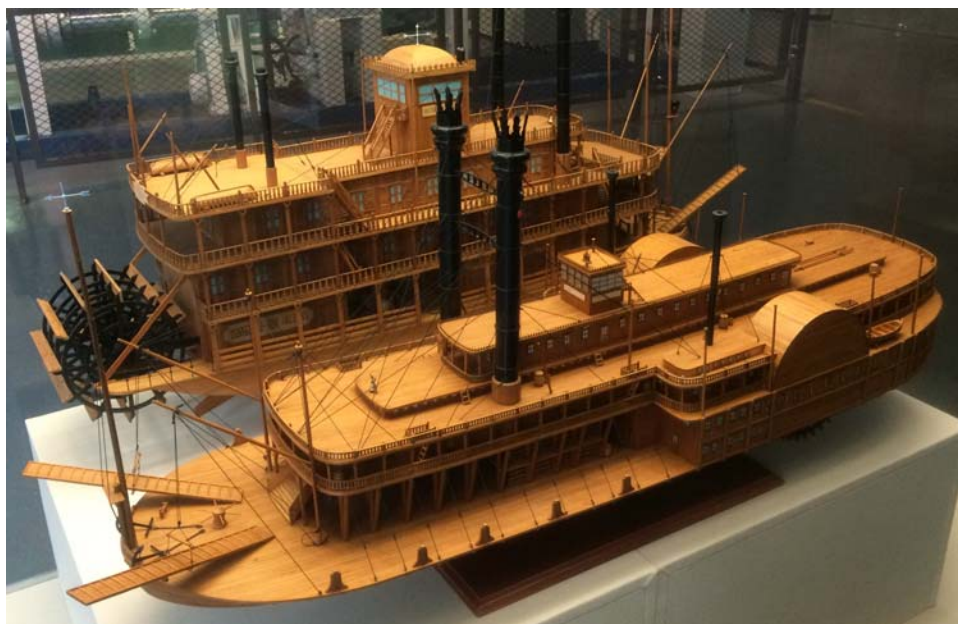
Figure 3: Models of two Chinese paddle steamers, a sidewheeler in the foreground and a sternwheeler in the background.
