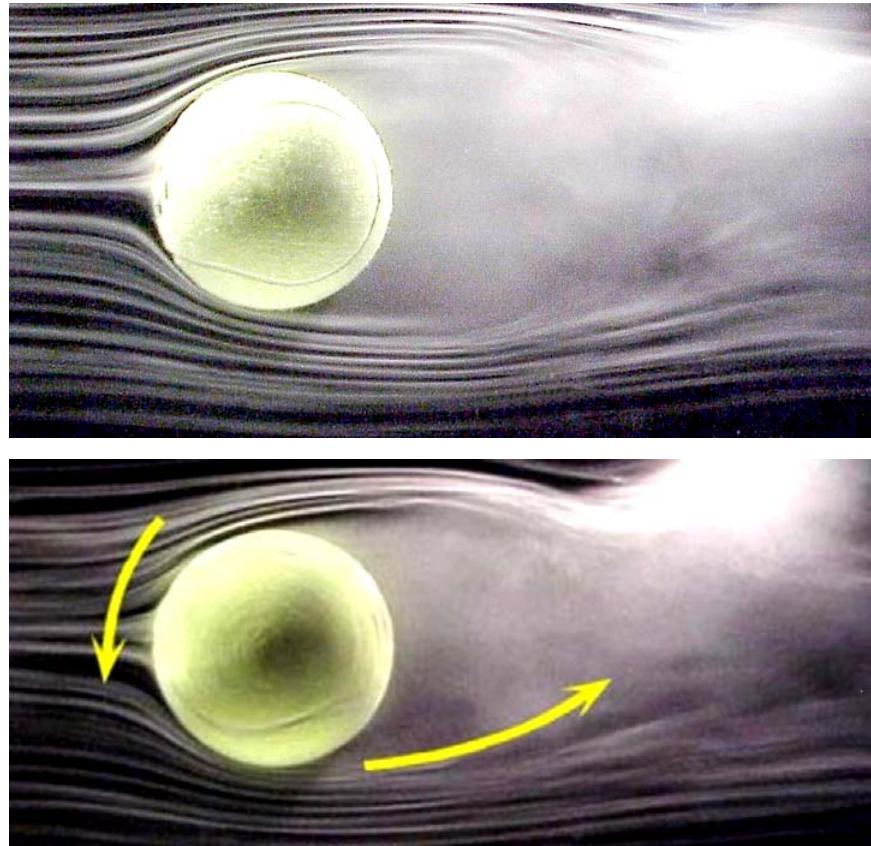
Figure 4: Flows around a non-rotating tennis ball at  $Re = 167,000$  (top) and around a tennis ball rotating anticlockwise (bottom).
