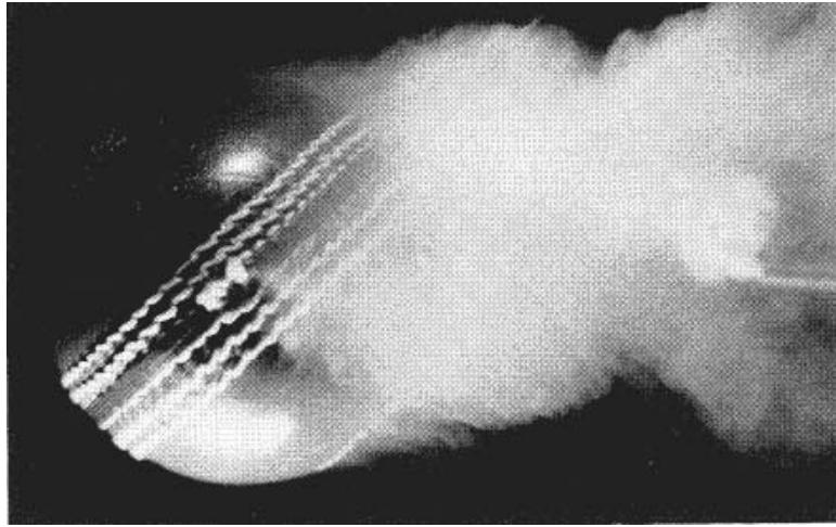
Figure 2: Flow around a cricket ball with  $U = 17m/s$ , seam angle =  $40^\circ$  and  $Re = 85000$ .
