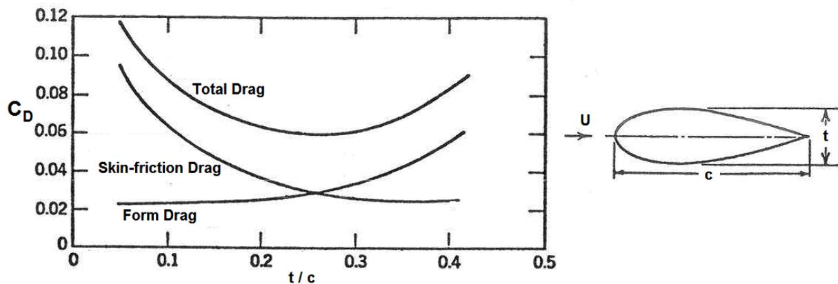
Figure 1: Coefficients of drag (based on frontal projected area) of a streamlined, symmetric strut (thickness,  $t$ , and chord,  $c$ ) as a function of the ratio,  $t/c$ . Shown are the  $C_D$  values for the form drag and the skin-friction drag as well as the total.
