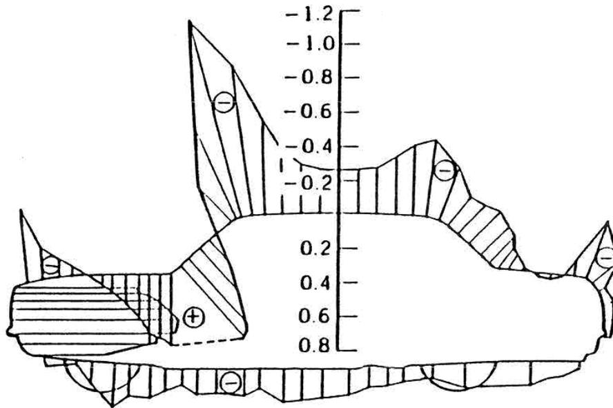
Figure 2: Typical pressure coefficient distribution on an automobile showing surface areas with pressures higher than upstream (+) and surface areas with pressures below upstream (-). The lengths of the vectors normal to the surface correspond to the coefficients of pressure shown on the scale.
