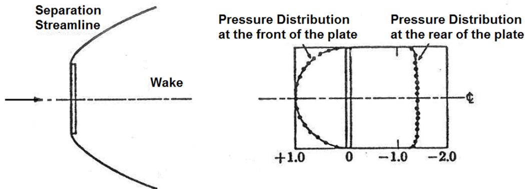
Figure 1: Flow and drag on a plate normal to a flow with the distributions of the coefficient of pressure on the front and rear shown on the right.
