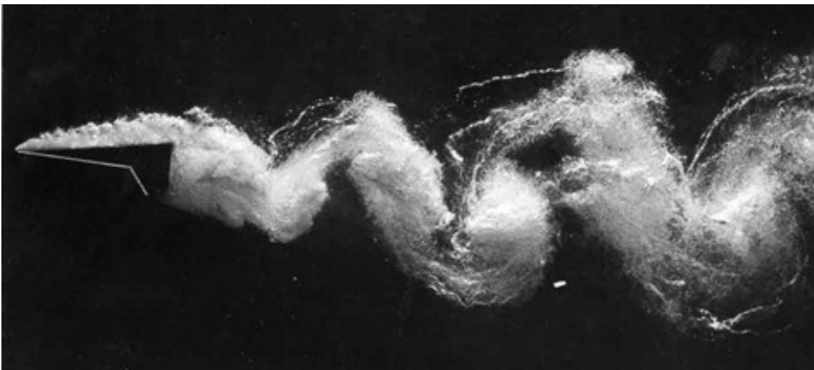
Figure 2: A cavitating vortex street behind a hydrofoil with a flap.
