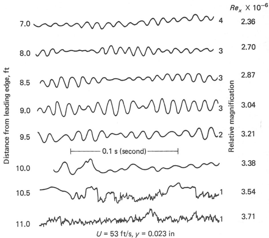
Figure 2: Unsteady velocity fluctuations with time at various longitudinal locations (distances from the leading edge on the left) in a transitioning boundary layer shown at various amplitude magnifications (shown on the right). The corresponding Reynolds numbers,  $Re_x$ , are also shown on the right. After Schubauer and Skramstad (1947).
