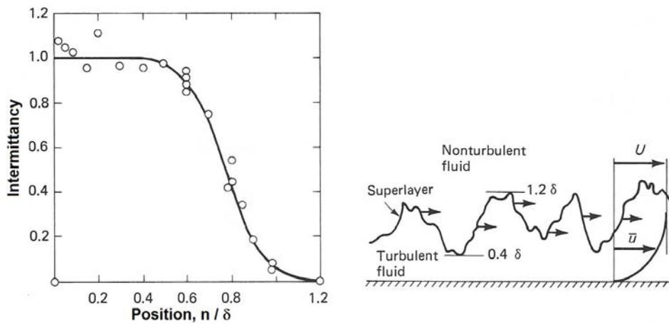
Figure 9: Intermittency in a turbulent boundary layer as sketched on the right and quantified in the graph on the right by the intermittency parameter. After Klebanoff (1955).
