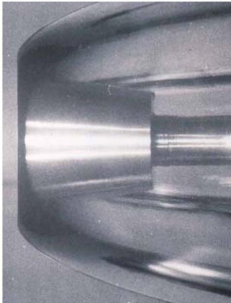
Figure 5: Flow of water past a disc headform showing no Tollmein-Schlichting waves or transition of the interfacial layer (Brennen (1970)).
