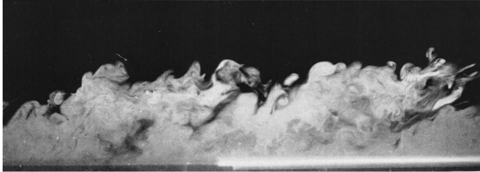
Figure 8: Visualization of a turbulent boundary layer on a wall at a point where the Reynolds number based on the momentum thickness is about 4000. After Falco (1977).
