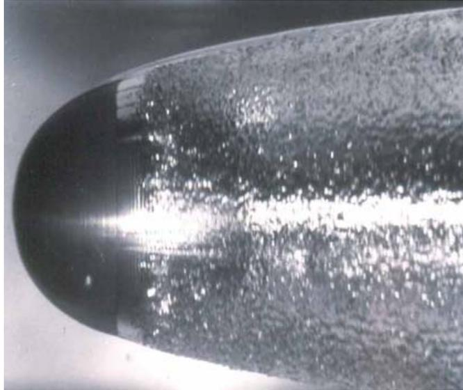
Figure 4: Flow of water past a spherical headform showing the growing Tollmein-Schlichting waves on the interfacial layer just after separation (Brennen (1970)).
