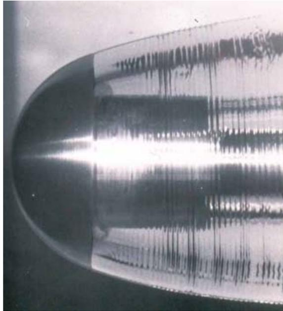
Figure 6: Flow of water past a spherical headform showing Tollmein-Schlichting waves whose growth is very limited (Brennen (1970)).
