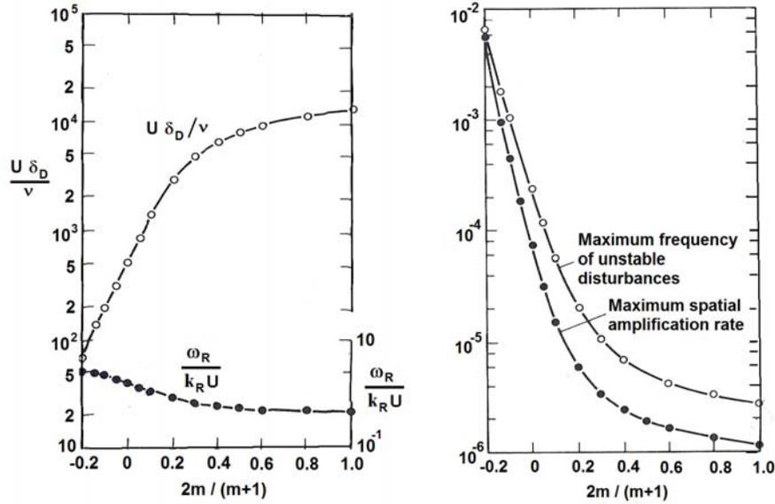
Figure 4: Spatial amplification data for the Falkner-Skan boundary layer velocity profiles. Left: values of the critical Reynolds numbers,  $U\delta_D/\nu$  (left scale), and the corresponding disturbance velocity,  $\omega_R/Uk_R$  (right scale), plotted against  $2m/(m+1)$ . Right: values of the maximum frequency of unstable perturbations,  $\omega_R\nu/U^2$ , and the maximum spatial amplification rates,  $-k_I\nu/U$ , as functions of  $2m/(m+1)$ . Adapted from Sherman (1990).
