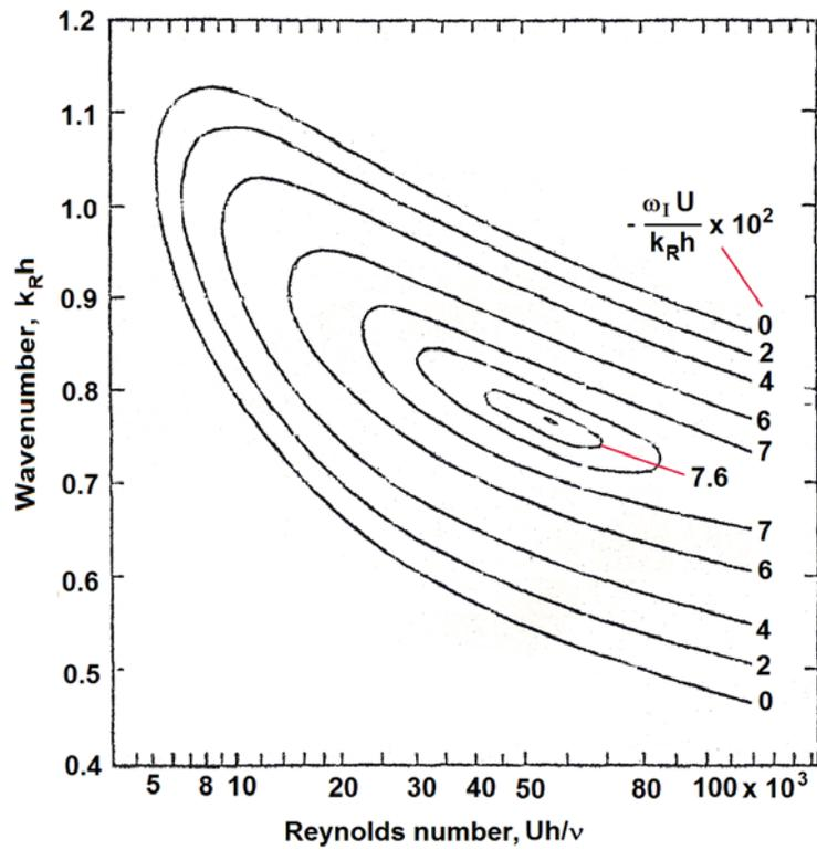
Figure 10: Spatial amplification for planar Poiseuille flow in a graph of the perturbation wavenumber,  $k_R h$ , plotted against the Reynolds number,  $Uh/\nu$ . Contours of several amplification rates,  $-\omega_I U/k_R h$ , are shown. Adapted from Shen (1954).
