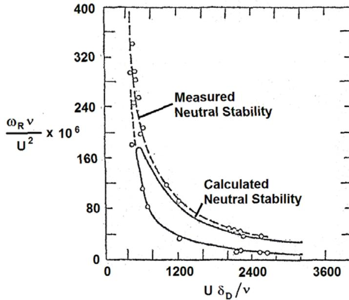
Figure 2: As Figure 1, comparing the calculated neutral stability boundary with experimental measurements. Adapted from Schlichting (1960).
