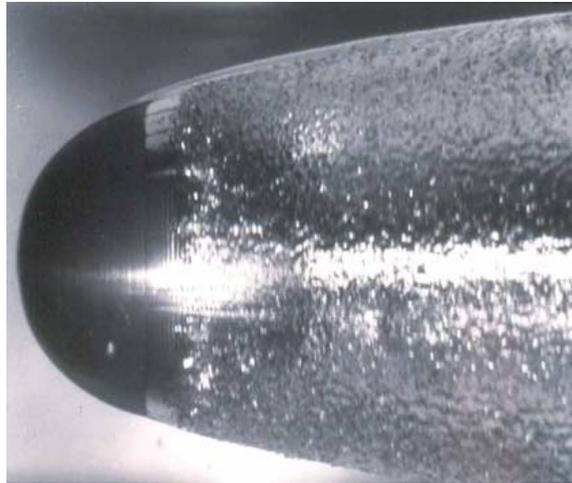
Figure 6: Flow of water past a spherical headform showing the growing Tollmein-Schlichting waves on the interfacial layer just after separation (Brennen 1970).
