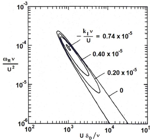
Figure 3: Spatial amplification for the Blasius boundary layer velocity profile in a graph of the perturbation frequency,  $\omega_R \nu / U^2$ , plotted against the surrogate distance parameter,  $\delta_D U / \nu$ , showing contours of several amplification rates,  $-k_I \nu / U$ , as indicated. Adapted from Jaffe *et al.* (1970); see also Sherman (1990).
