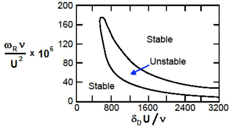
Figure 1: Neutral stability boundary ( $k_I = 0$ ) for the Blasius boundary layer velocity profile in a graph of the perturbation frequency,  $\omega_R \nu/U^2$ , plotted against the surrogate distance parameter,  $\delta_D U/\nu$ .
