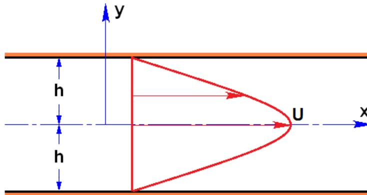
Figure 9: Planar Poiseuille flow between two flat plates.
