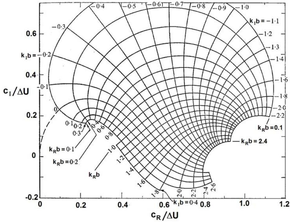
Figure 8: General amplification chart for the spatial or temporal stability of an interfacial boundary layer with a free surface in a graph of the imaginary wavenumber,  $c_I/\Delta U$ , plotted against  $(U - c_R)/\Delta U$ . Contours of real and imaginary wavenumbers,  $bk_R$  and  $bk_I$  are shown. Adapted from Brennen (1970).
