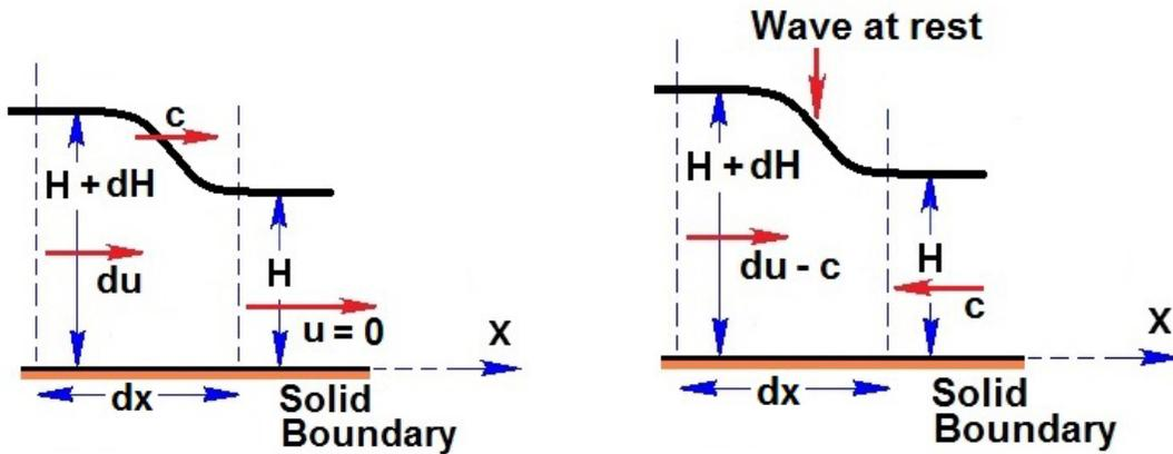
Figure 1: Small disturbance propagation: Left: In frame of right-hand fluid. Right: In frame fixed in wave.
