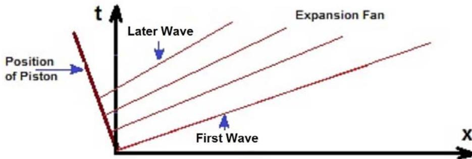
Figure 2: Space/time diagram for an expansion wave in open channel flow.
