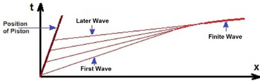
Figure 3: Space/time diagram for a compression wave in open channel flow.
