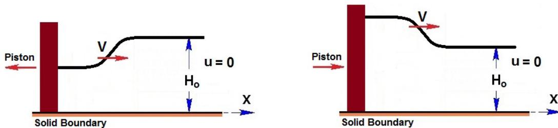
Figure 1: Conceptual formation of an expansion wave (left) and a compression wave (right) in an open channel flow.
