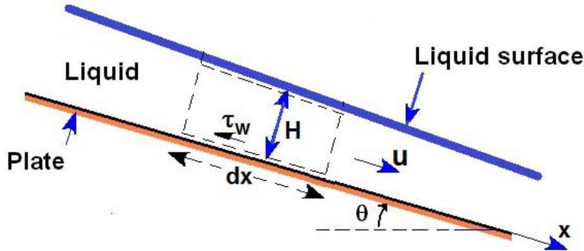
Figure 1: Open channel flow down an inclined plane with friction,  $\tau_w$ .
