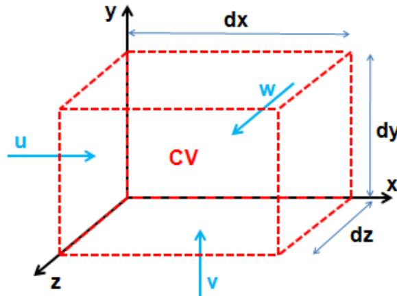
Figure 1: Infinitesimal Eulerian control volume.
