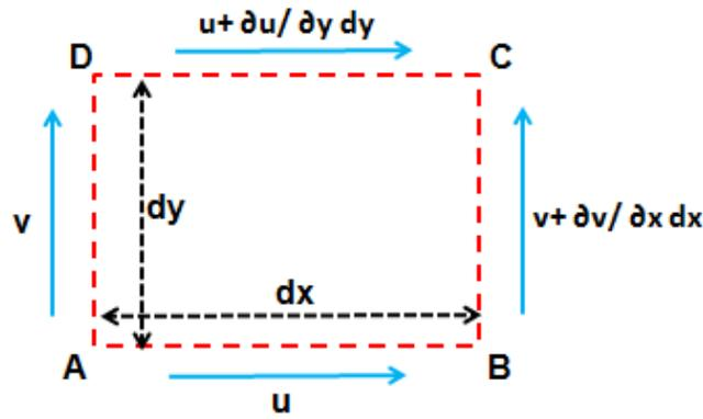
Figure 2: Circulation around an infinitesimal element.
