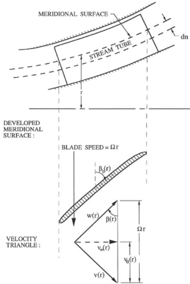
Figure 2: Developed meridional surface and velocity triangle.
