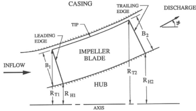
Figure 1: Cross-sectional view through the axis of a pump or turbine rotor.
