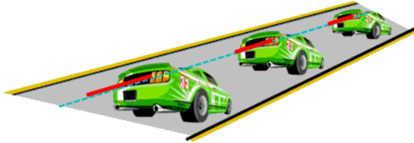
Figure 2: Streamline (blue dashed line) from short time exposure involving multiple cars.
