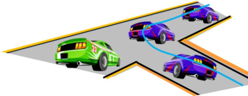
Figure 4: Streakline (blue) connecting all cars passing through a particular point.
