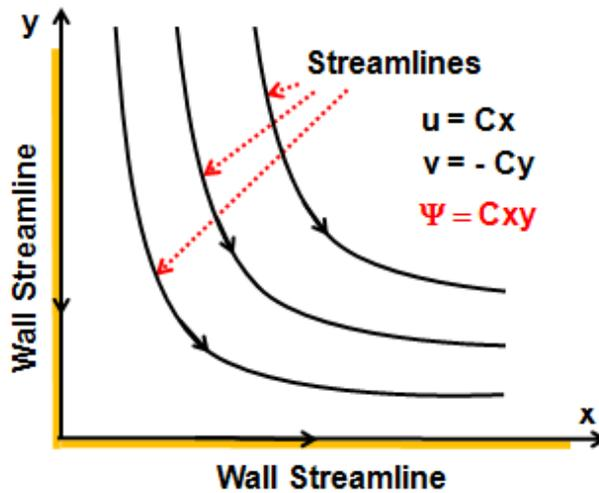
Figure 5: Flow in a rectangular corner with walls.
