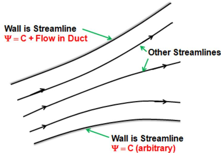
Figure 1: Streamlines in a duct.
