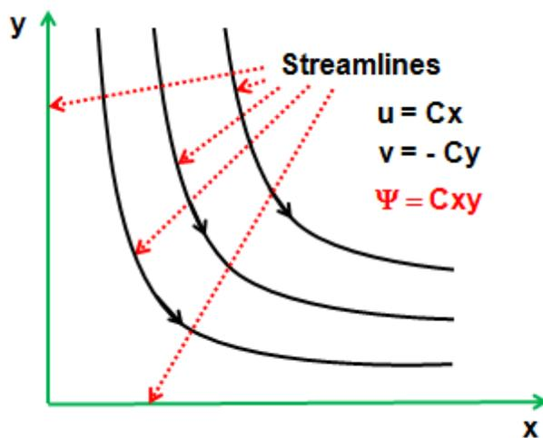
Figure 4: Flow in a rectangular corner.
