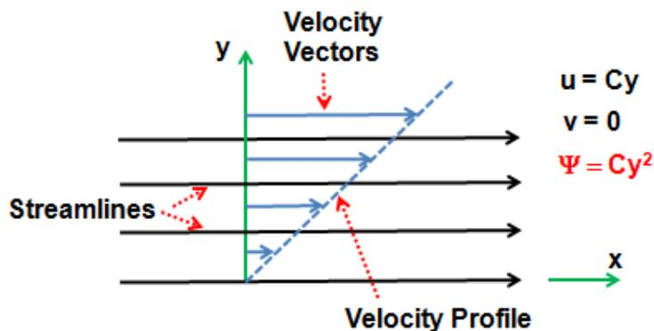
Figure 3: Shear flow in the  $x$  direction.
