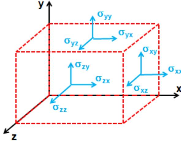
Figure 1: Differential element indicating the nine stresses.
