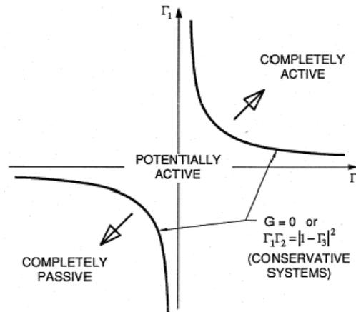
Figure 1: Schematic of the conditions for completely active, completely passive and potentially active components or systems.
