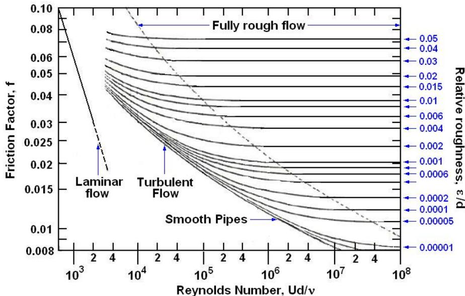
Figure 1: Moody diagram for the pipe friction factor as a function of the pipe Reynolds number.
