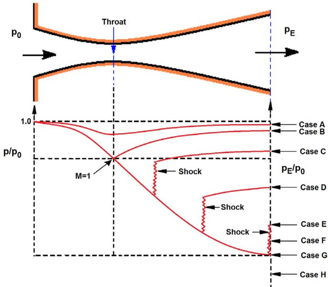
Figure 1: A de Laval nozzle with the pressure distributions for various exit pressures.
