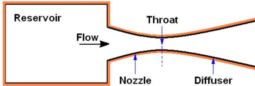
Figure 1: Schematic of general converging/diverging nozzle.
