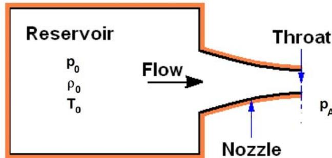
Figure 3: Schematic of a nozzle ejecting to atmosphere.
