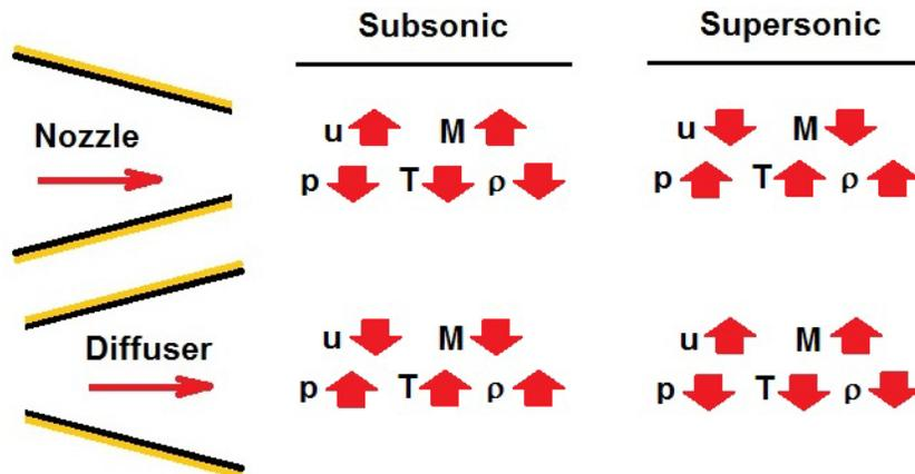
Figure 2: Variations of flow properties in a nozzle and a diffuser.
