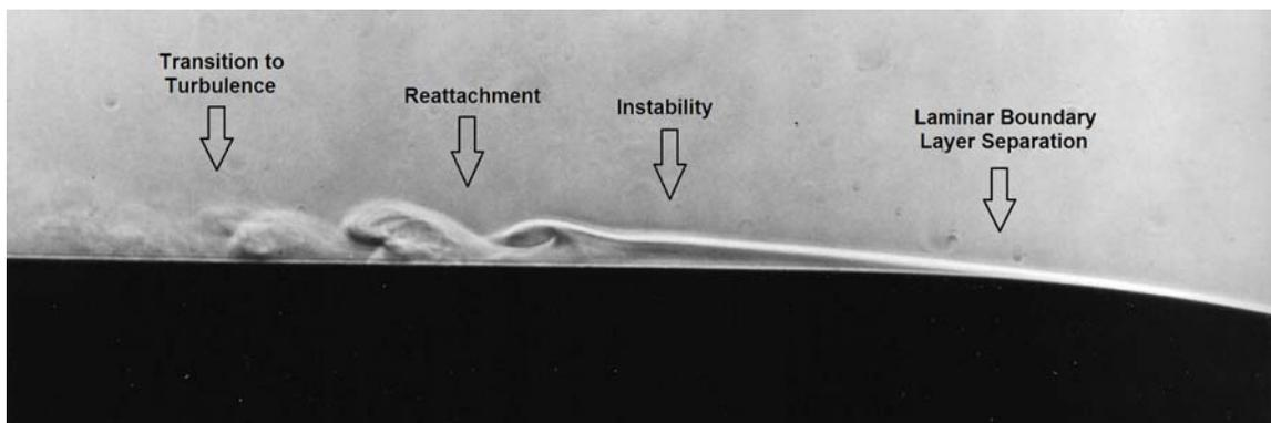
Figure 2: Shadowgraph photograph taken by V. Arakeri of the development of the boundary layer flow on the surface of an object in a water tunnel. The flow is from the right to the left.
