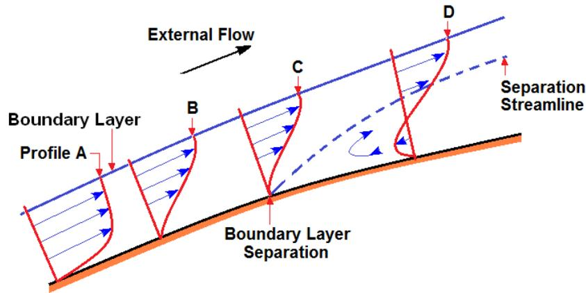
Figure 1: Sketch demonstrating the development of a laminar boundary layer in a decelerating external flow.
