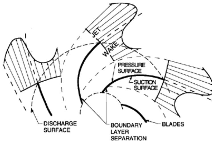
Figure 1: A sketch of actual discharge flow from a centrifugal pump or compressor including the alternating pattern of jets and wakes resulting from flow separation from the suction surfaces.
