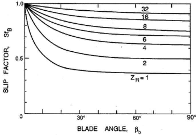
Figure 3: The Busemann slip factor,  $Sf_B$ , plotted against the blade angle,  $\beta_b$ , for various numbers of blades,  $Z_R$ . The results shown are for radial cascades of infinitely thin logarithmic spiral blades with solidities,  $s > 1.1$ . Adapted by Sabersky, Acosta and Hauptmann (1989) and Wislicenus (1947) from Busemann's (1928) theory.
