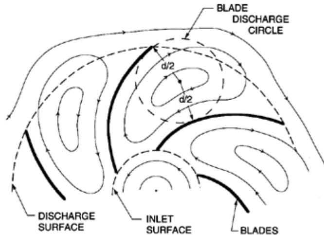
Figure 2: A sketch of the displacement component of the inviscid flow through a rotating radial cascade.
