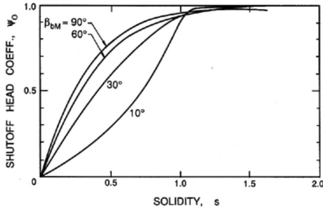
Figure 3: The performance parameter,  $\psi_0$ , as a function of solidity,  $s$ , for flat plate cascades with different blade angles,  $\beta$ . Adapted by Wislicenus (1947) (see also Sabersky, Acosta and Hauptmann 1989) from the potential flow theory of König (1922).
