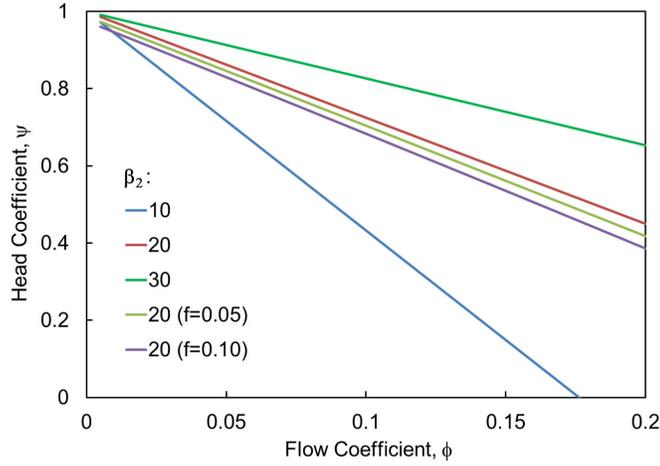
Figure 2: Calculated head/flow characteristics for some linear cascades.
