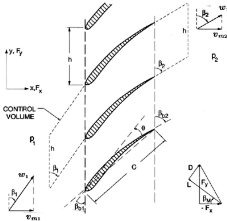
Figure 1: Schematic of a linear cascade showing the blade geometry, the periodic control volume and the definition of the lift,  $L$ , and drag,  $D$ , forces on a blade.
