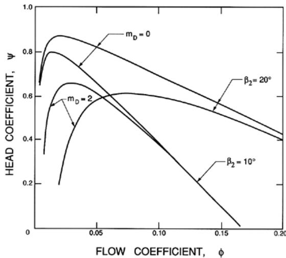
Figure 4: Calculated head/flow characteristics for a linear cascade using blade drag coefficients given by equation (Mbc18) with  $C_{D0} = 0.02$ . The corresponding characteristics with  $C_{D0} = m_D = 0$  are shown in figure 2.
