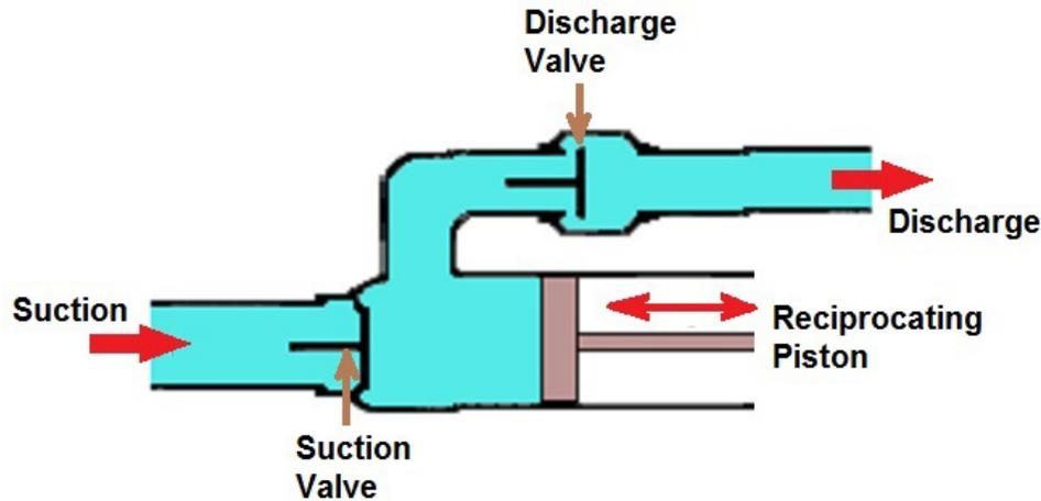
Figure 1: Schematic of a simple positive displacement pump.
