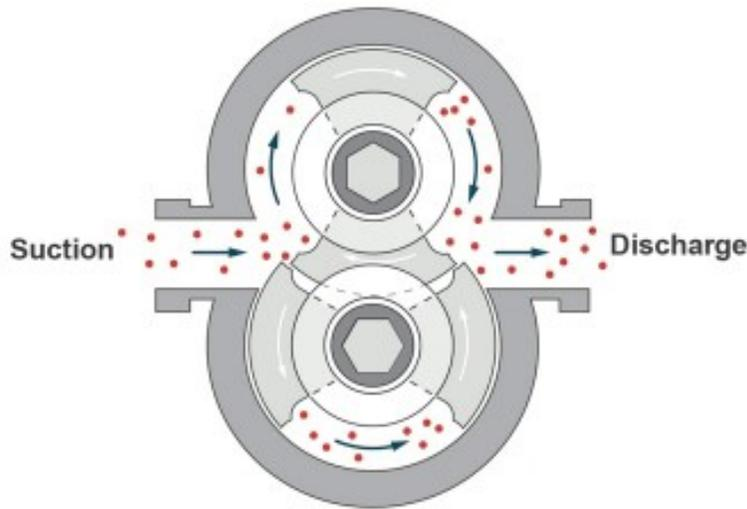
Figure 4: Geometry of the AMPCO ZP1 positive displacement pumps.
